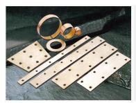
TETF01 self-lubricating bearings are optimised on the basis of TE80 bimetallic bushings. The bearing offers excellent anti-friction properties. It works even when no oil is used. The graphite in the bushings provides excellent protection of the shaft against seizure when working in high temperatures or without oil lubrication. The bushings can be used for guiding rubber tyre moulds and parts of water turbines that slide at high speed.
