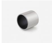
TEP4 consists of a steel backing with sintered porous bronze alloy, PTFE and polymer coating. TEP4 is lead-free and has good anti-wear, anti-fatigue, anti-punching and high bonding performance. it can now be applied as a substitute for TED1 and TEP1 type bearings.
