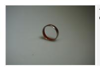
TEMUT is a three layer bearing. TEMUT is made with a steel back, sintered porous bronze powder layer and a rolled misture of PTFE and environment-friendly polymer. Suitable for a higher speed rotation.
