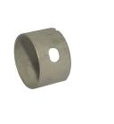
TEHTC steel bushing is made of low-carbon steel with a carbonitriding process. So the working surface formed a high hardness wear layer. This bushing has many advantages, like dimensional stabilisation, hardness uniform, high wear resistance, high tenacity, impact resistance, long service life, etc. It can be used in engine rocker parts.
