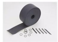
TEFD02 soft strip is based on PTFE and filled with graphite and other lubricants. It is made by pressing and sintering. This material has good elasticity, a low friction coefficient, and high wear resistance. It most commonly fits to be used along with a metal base. Providing excellent friction and wear performance, it can be used as a piston for shock absorber and oil cylinder. It is widely used in many car brands, including Volkswagen, Buick, etc.
