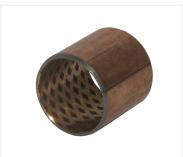
TEBRM95 is based on bronze and embedded with solid lubricants. Because it is made of bronze, which performs well in terms of elongation, it can be processed into a wrapped bushing with thin wall thickness. In addition, the embedded lubricant is ideal for lubrication, and the bushing can be used in car transmission shafts and other circumstances without oil lubrication.
