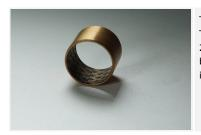
TEBRM85 is a kind of steel-lead bronze alloy based bearing embedded with a particular composition of solid lubricants. The spiral diamond embedded in solid oil ensures high strength and high load capacities. With a lubrication area of 25% on the bearing surface, the bushing shows improved performance in terms of good lubrication and anti-wear. This bearing type is widely used in gearboxes for automobiles, generators, cranes and machines for the metallurgical industry.
