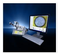
Manufacturers and users of hard coatings are often confronted with the problem of the measurement of the thickness of coatings. AsecTribo has created a new and innovative instrument called CALOTESTER fully equipped with all items needed for measuring thickness of coatings, at your fingertips: programmed spherical abrasion controlled by microprocessor. Microscope for measurement of abraded coatings and a calculator to supply the results of thickness automatically.
