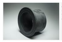
ASRS20 bearing materials are reinforced woven polymers specially developed for high loads and smooth running. The material contains an ideal concentration of graphite that provides excellent performance in conditions where reduced friction and wear are required. ASRS20 has good wear resistance and is suitable for use in dry, wet and lubricated conditions. ASRS20 has a low coefficient of friction, is resistant to edge loading and does not rapidly swell in water.
