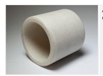
ASRS10 is a composite of reinforced polyester resin with synthetic fiber and micro self-lubricating powders. This mix results in good wear resistance and low friction and works very well in oilles or low-oil conditions.
