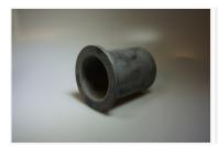
The ASN988 material is recommended for use in high load bushings and bearing applications. The material offers market-leading frictional properties for composite materials. ASN988 is a high load composite bearing material made from specially manufactured synthetic fabric reinforcement employing a composite construction process impregnated with thermosetting resins. Solid lubricant fillers are added, making them suitable for dry-running applications. The product has a dark grey colour.
