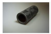
The ASN901 material is suitable for use in high load bushing and bearing applications. The material offers marketleading frictional properties for composite materials. ASN901 is a high-load composite bearing material made from specially manufactured synthetic fabric reinforcement using a composite construction process impregnated with thermosetting resins. Solid lubricant fillers are added, making them suitable for dry-running applications. The product has a dark grey colour.
