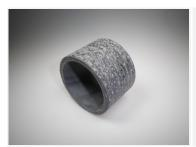
The ASN788 material is recommended for use in high load bushings and bearing applications. The material offers market leading frictional properties for composite materials. ASN788 is a high load composite bearing material made from specially manufactured synthetic fabric reinforcement using a composite construction process impregnated with thermosetting resins. Solid lubricant fillers are applied, making them suitable for dry-running applications. The product has a dark grey colour.
