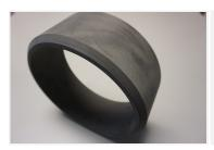
ASN605 composite bearing material is made from a custom-manufactured synthetic fabric reinforcement impregnated with thermosetting resins and solid lubricant fillers to improve dry running capability. ASN605 has a dark grey colour.
