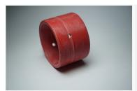
ASN422 material is specifically intended for use in high load bushing and bearing applications. ASN422 is a high load composite bearing material manufactured from synthetic fabric reinforcement impregnated with a thermosetting resin. Solid lubricant fillers are used to reduce friction. The product has a red colour.
