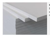
Mineral bonded, lightweight non-combustible steam-cured calsium silicate board with moisture resistant properties. Suitable for the fire-resistant protection of steel columns and beams and the realization of wall, shaft wall and ceiling constructions with a fire separating function, which must also meet certain requirements with regard to moisture resistance.
