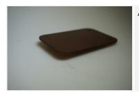
Al PF CP 207 is a phenolic strengethened paper based composite material
