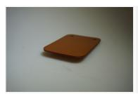
Al PF CP 206 Is a construction material for mechanical, electrotechnical and high-frequency purposes. Resistant to tropical conditions, where high humidity is expected. Suitable as high-frequency insulation thanks to low dielectric dissipation factor.
