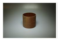
Al PF CC 24 for mechanical applications. Impact-resistant, noise-reducing, wear-resistant material. Well suited as a lowfriction material. High wear resistance in aggressive and dust-filled environments. Can be lubricated with water, oil or grease. Examples of applications are ball-bearing cages for spindle bearing and guide rings for hydraulic cylinders. Can be used, in particular, for mechanical applications where fine tolerances and smooth surface finish are required.
