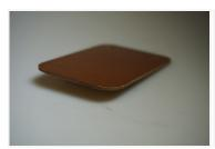
AI PF CC 203 is reinforced with a finer cotton fabric than AI PF CC 201. Also, well suited in particular for small components which are subject to mechanical load and wear. Can be machined to finer tolerances and smoother surface finish than AI PF CC 201.
