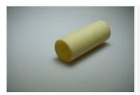
AI MF GC 201 Is suitable for mechanical and electrical applications. Arc-resistant and tracking-resistant material. Good flame resistance. Self-extinguishing. Halogen-free. Lower high-voltage values and insulation resistance than other AI EP GC and AI PF GC.
