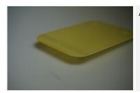
AI MF CC 201 is a melamine strengthened- cotton cloth -based composite material
