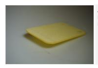
AE IP PC 301 is characterized for being strong and tough. It is also the lowest in welling in water and has an incredibly low water absorption. AEIPPC301 is high chemical resistance, e.g., to SF6 gas. When there is SF6 gas used as an insulation medium AEIPPC301 is suitable for high/voltage circuit breakers.
