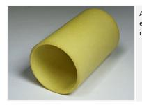
Al EP GC 21 Has particularly good electrical and mechanical properties. Extremely high mechanical strength. Retains electrical properties at high air humidity. High resistance to chemicals. Engineering and insulation material in large rotating electrical machines and insulation cylinders in dry transformers.
