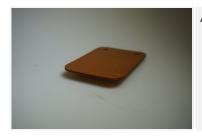
AI EP CP 201 is a composite with paper as a base, strengethened with epoxy
