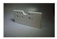
AlDuratecXP is a asbestos fibre free glass fibre reinforced calcium silicate large sized board. These boards are made in a density of 1800 kg/m3. Ideal suited for replacing asbestos containing materials in all industrial applications. The material is non-brittle and electrically inert.
