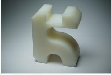
ASXUELS has a 50% reduce of stiffness and yield strength. But the important properties of POM-C remains unchanged.
