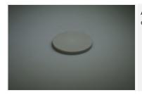
AE900XT Can operate at a higher speed while exhibiting reduced wear, also the "slip-stick" behavior is reduced. This can be achieve by using a solid lubricate.
