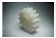
AE1100 is a cast polyamide 6 heavy duty, high impact, and chemical resistant material for bigger parts. It has high wear resistance at low and middle speeds and performs especially well under harsh conditions such as contact with sand or dust. Due to its balaced mechanical properties and its exceptional machinability it is the ideal engineering material for a wide range of applications.
