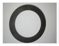
Asbestos-free, rigid molded friction material based on graphite and phenolic resins as bonding system, containing short fibers, friction lubricants and fillers. Suitable for industrial applications, continuous brake, brake calipers, friction rings, brake pads, torque limititer. Recommended friction surface: pearlitic grey cast iron.
