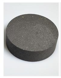
It's a black rigid friction material based on graphite with a medium low friction coefficient. Phenolic resins is used as a bonding system with short fibers, friction lubricants and fillers. AB3420 is cured and suitable for bonding and reviting.
