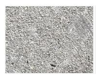
Asbestos-free, pressed composite friction material containing metallic components. AB3160 is based on phenolic resins with NBR rubber bonding system, containing short fibers, organic components, friction modifiers, metallic particles, and fillers. AB3160 is suitable for dry and oil immersed applications. AB3160 is not abrasive to the counter face material and is silence in operation. AB3160 is resistant to high pressure. It has low wear rate even at high temperatures.
