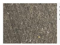
Asbestos-free, pressed composite friction material containing metallic components. AB3080 is based on phenolic resins with NBR ruber bonding system, containing short fibers, organic components, friction modifiers, metallic particles and fillers. AB3080 is suitable for dry and oil-immersed applications. AB3080 is not abrasive to the counter face material and is silence in operation, It is resistant to high pressures and has low wear rate even at high temperatures.
